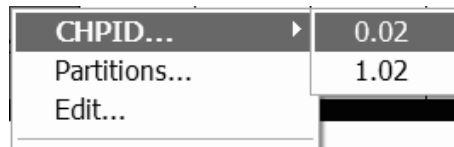
Figure 12. Context menu of a spanned CHPID in a vertical processor view
